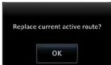
Figure 4-51 Touch OK to Replace the Existing Active Flight Plan
