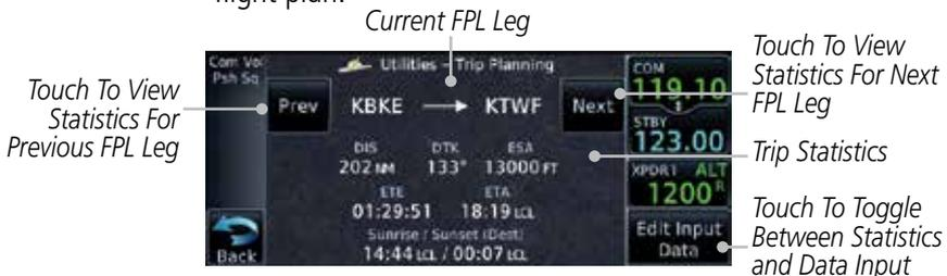
**Figure 14-26 Utility Trip Planning Page Computed Data View Of Next Waypoint (Flight Plan Mode)**
