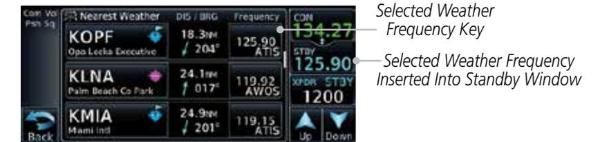
Figure 12-23 Nearest Weather Station Selected Frequency
