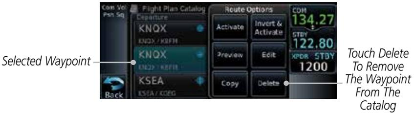
Figure 4-59 Select a Flight Plan from the Catalog
