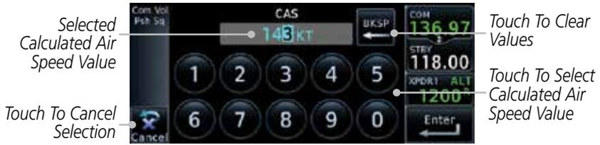
**Figure 14-43 Select Calculated Air Speed Value**
