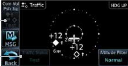
**Figure 9-2 Traffic Test Mode**
