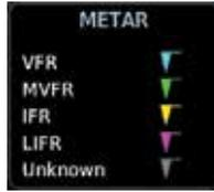
**Figure 11-65 Connex Weather - Graphic METARs and Legend**
