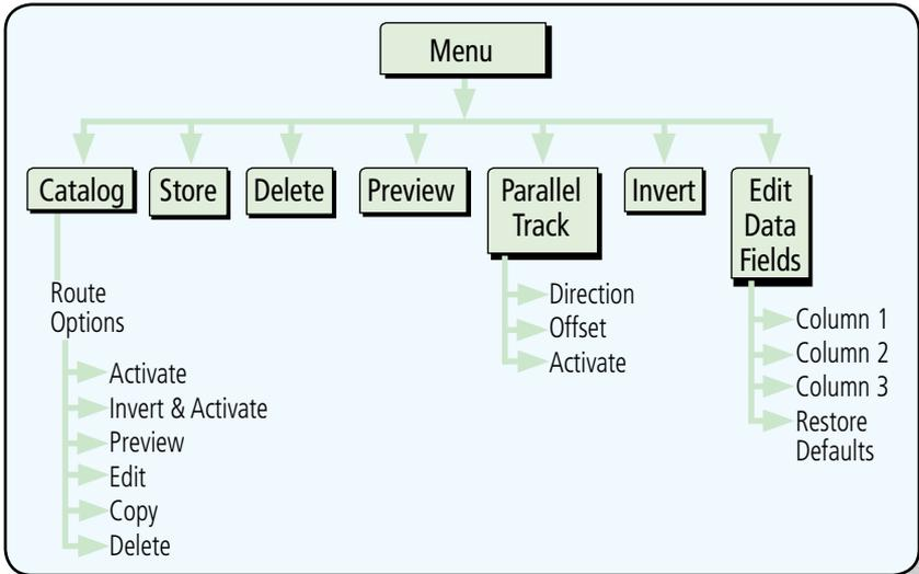
Figure 4-41 Flight Plan Menu Functional Diagram
