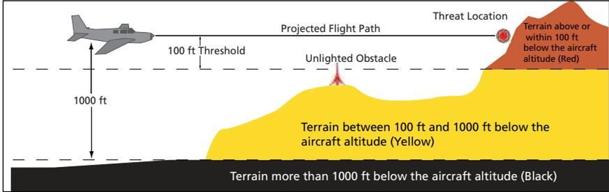
Figure 10-6 Terrain Altitude/Color Correlation for Terrain Proximity
