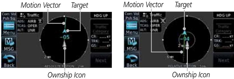
**Figure 9-15 Comparison of Absolute and Relative Motion Vectors With a Single Target**
