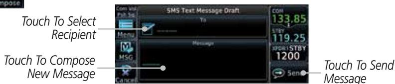
**Figure 13-23 Compose a New SMS Text Message**
