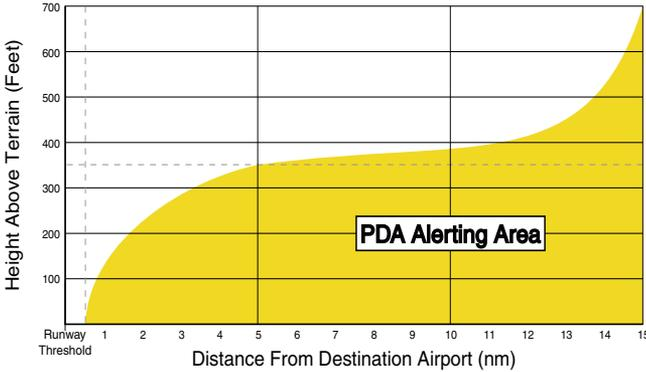
**Figure 10-35 PDA Alerting Threshold**
