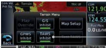
*Touch To Toggle TAWS Inhibit. TAWS Inhibited shown.*
