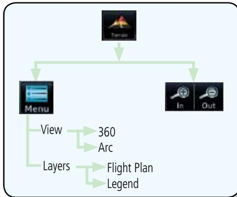
Figure 10-1 Terrain Proximity Page Functional Diagram
