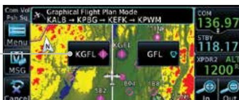
Figure 8-42 Select the Desired Waypoint From Multiple Waypoints
