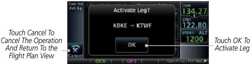
Figure 4-10 Active Flight Plan Activate Leg Option
