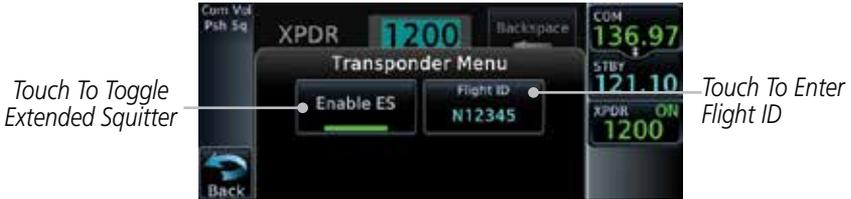
Figure 2-16 Transponder Menu With Extended Squitter Capability
