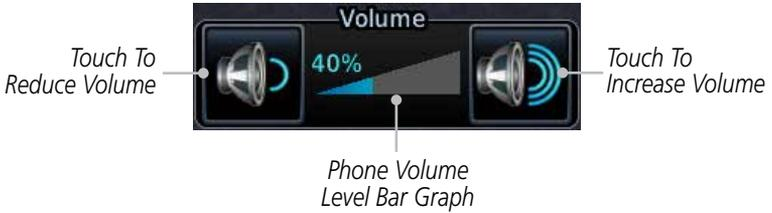
**Figure 13-20 Select Soft Keys for Phone Volume Adjustment**
