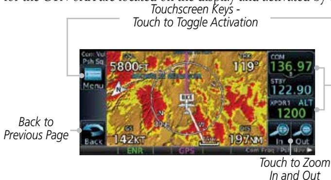
Figure 1-17 On-Screen Keys and Active Display Areas
