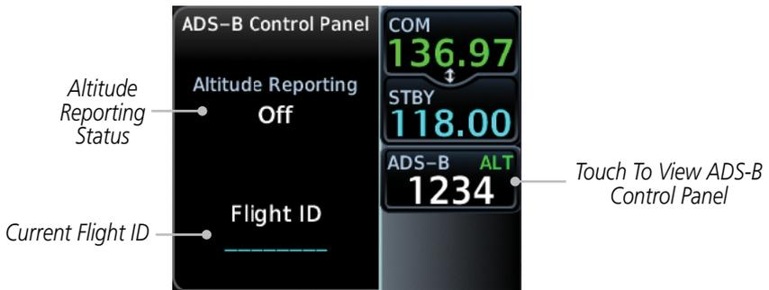
Figure 2-13 ADS-B Control Panel
