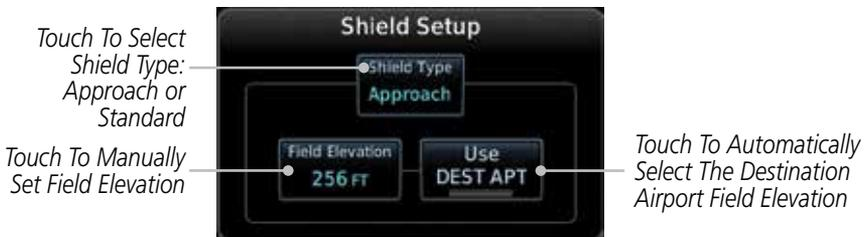
**Figure 9-34 TCAD 9900BX Shield Setup for Approach**
