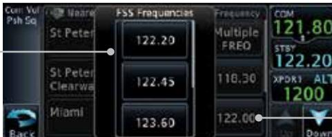
Selected FSS Frequency Inserted Into Standby Window
