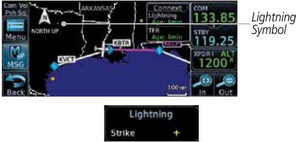
Figure 11-63 Connex Data Link Lightning and Legend
