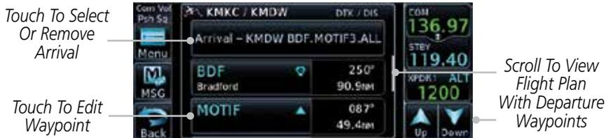
Figure 6-14 Flight Plan With Arrival Loaded
