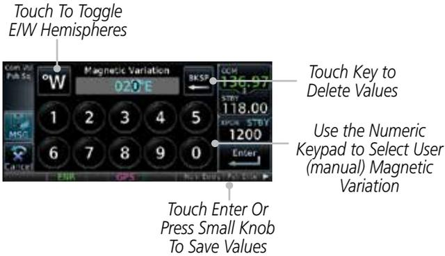
**Figure 15-55 Numeric Keypad for Setting Manual Magnetic Variation**
