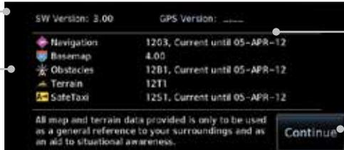
Check To Ensure Required Databases Are Present And Current
