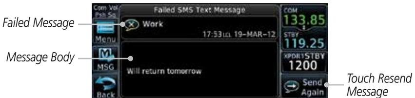
**Figure 13-26 Resend a Failed SMS Text Message**
