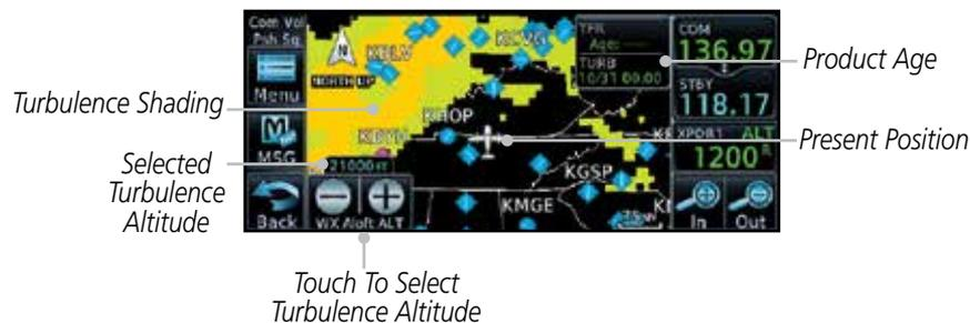
Figure 11-41 Turbulence
