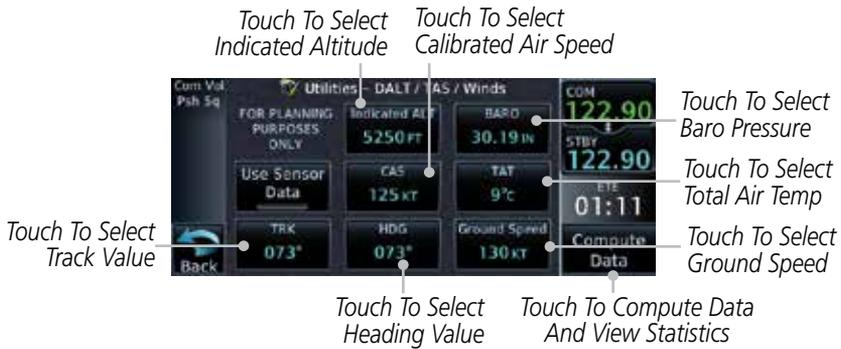
**Figure 14-39 Utility DALT/TAS/Winds Page Using Manually Entered Data**
