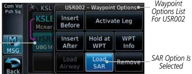
**Figure 4-28 Active Flight Plan with Load SAR Option**
