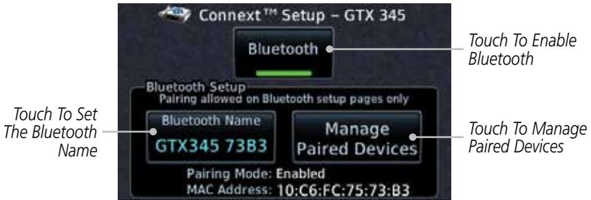
**Figure 15-67 Connex Setup for GTX 345**
