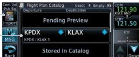
**Figure 4-72** Catalog for SD Card Flight Plan Import
