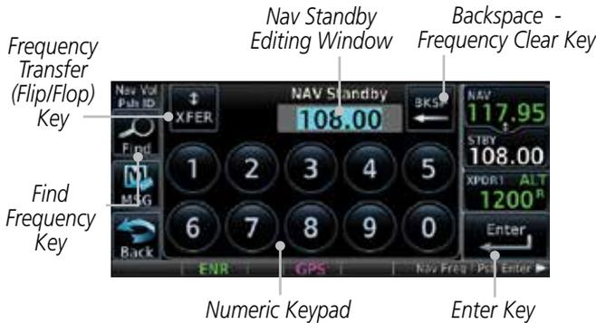
**Figure 3-6 Nav Standby Frequency Numeric Keypad**
