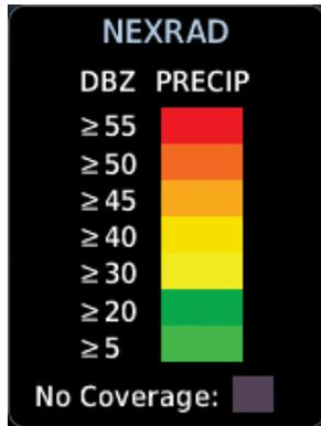
**Figure 11-70 FIS-B Weather Precipitation Legend**
