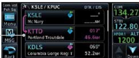
Figure 4-13 New Waypoint Is Inserted Before the Selected Waypoint
