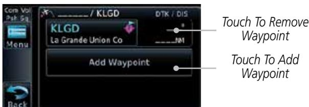
Figure 4-2 Create New Flight Plan
