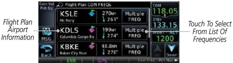
Figure 3-14 Flight Plan Frequency List
