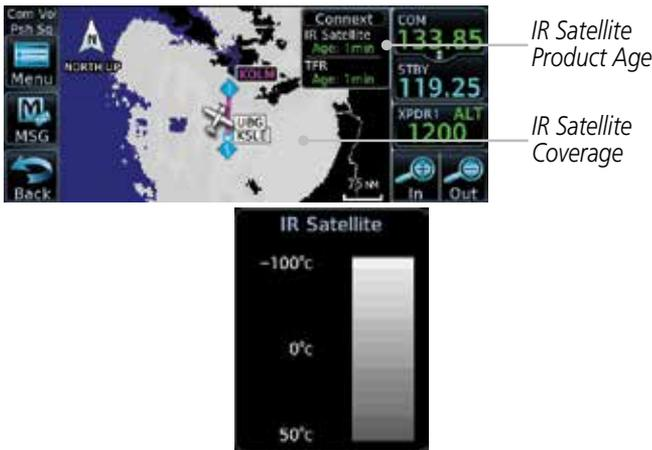
Figure 11-64 Connex Infrared Satellite Data Map Display and Legend
