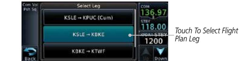
Figure 14-35 Select Flight Plan Leg
