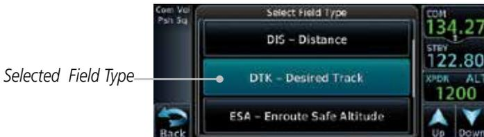
Figure 4-48 Flight Plan Data Fields List
