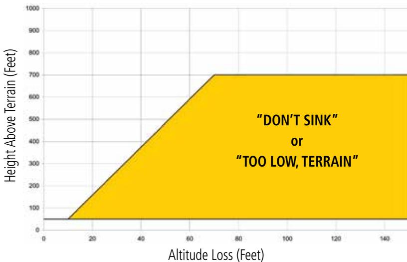
Figure 10-15 Negative Climb Rate (NCR) Altitude Loss
