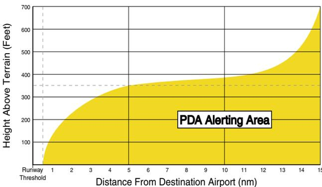
**Figure 10-13 PDA Alerting Threshold**
