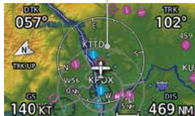
Figure 8-25 Display of Smart Airspaces (Airspace Borders Grayed)
