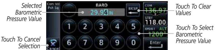
**Figure 14-42 Select Barometric Pressure Value**
