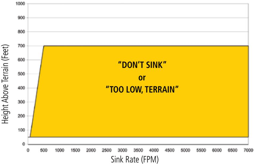
Figure 10-43 Negative Climb Rate (NCR) Sink Rate
