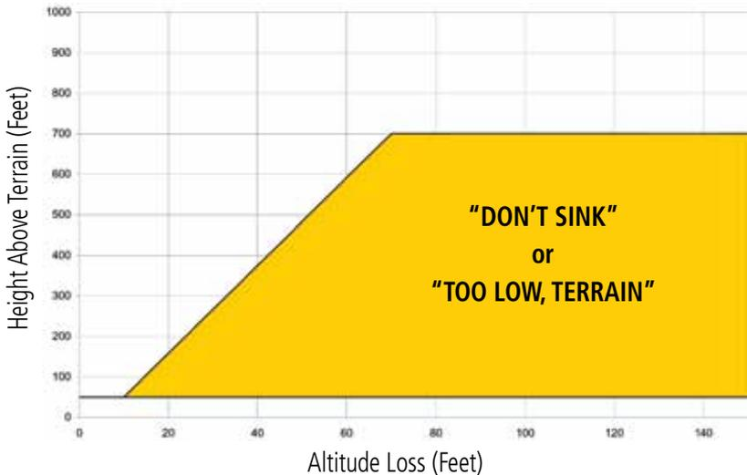
**Figure 10-42 Negative Climb Rate (NCR) Altitude Loss**
