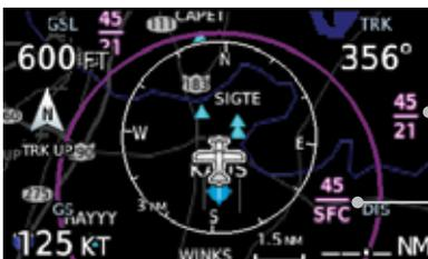
**Figure 8-24 Display of Airspace Labels**
