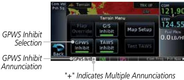
Figure 10-45 GPWS Inhibit Annunciation
