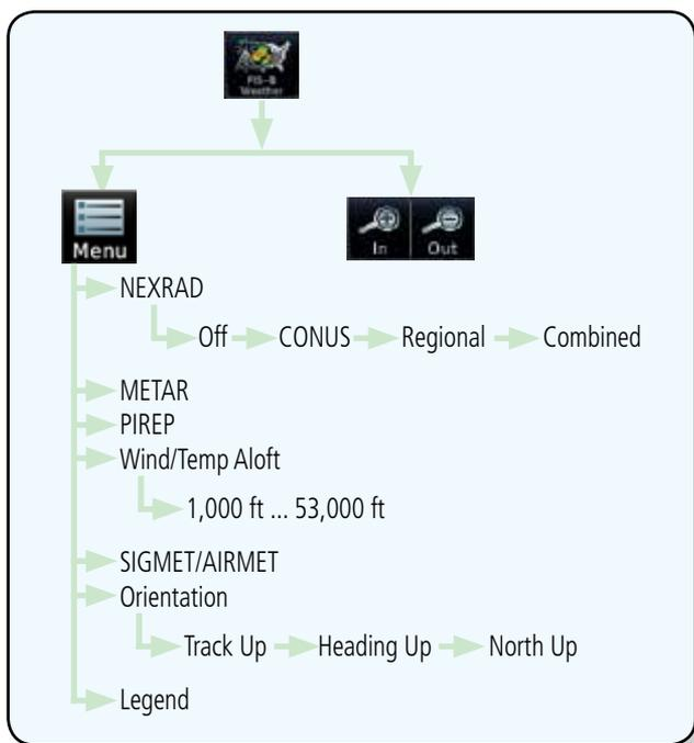
**Figure 11-71 FIS-B Weather Functional Diagram**
