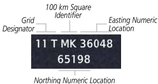
Figure 15-57 MGRS Position Format Detail
