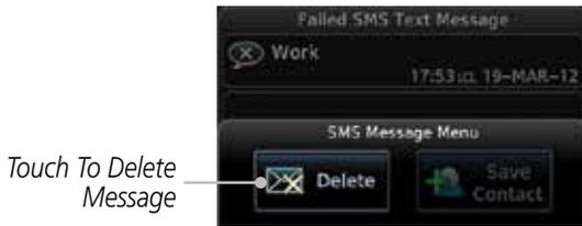
Figure 13-27 Delete a Failed SMS Text Message
