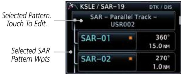
Figure 4-29 SAR Pattern Waypoints in the Flight Plan
