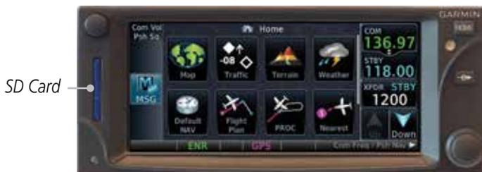
**Figure 18-1 SD Card Database Location**
