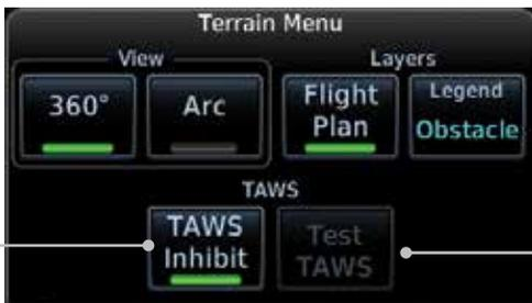
Figure 10-9 TAWS-B Alerts Inhibited Selected
