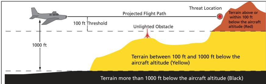
Figure 10-27 Terrain Altitude/Color Correlation for TAWS-A
