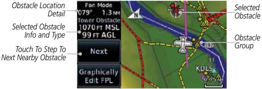
Figure 8-22 Point Obstacle Detail
