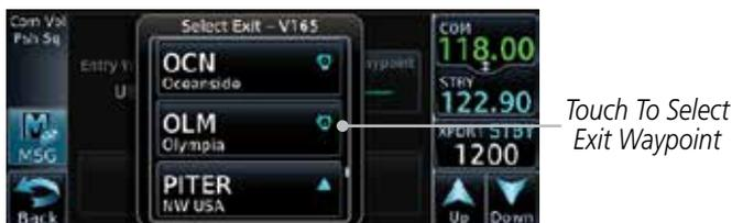
Figure 4-21 Select an Exit Waypoint for the Airway
