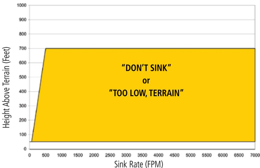
Figure 10-16 Negative Climb Rate (NCR) Sink Rate
