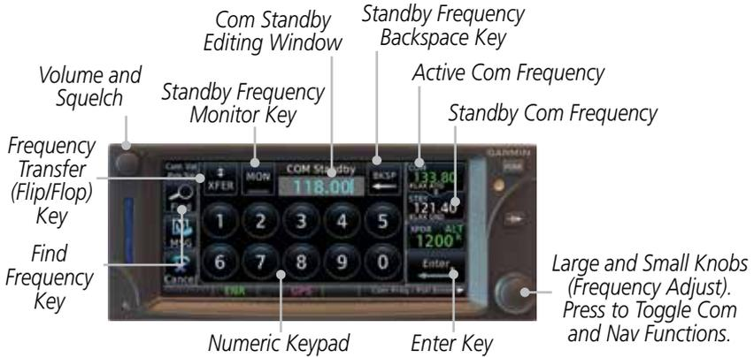
Figure 1-20 Com Radio Frequency Selection Page
