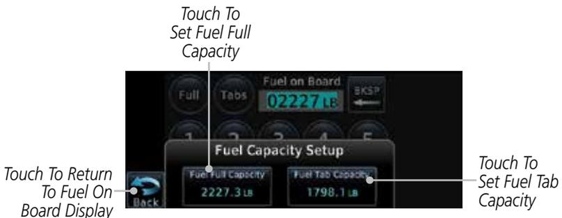
Figure 1-14 Fuel Capacity Setup Page
