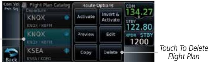
Figure 4-57 Select Flight Plan from the Catalog to Delete
