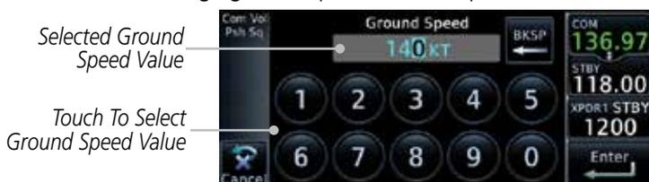
Figure 14-32 Selecting Ground Speed
