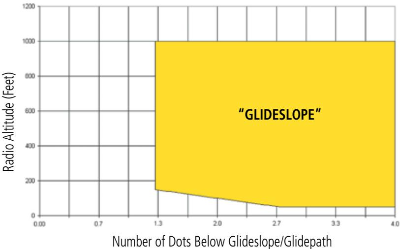
Figure 10-44 Excessive Below Glideslope/Glidepath Deviation Alert Criteria
