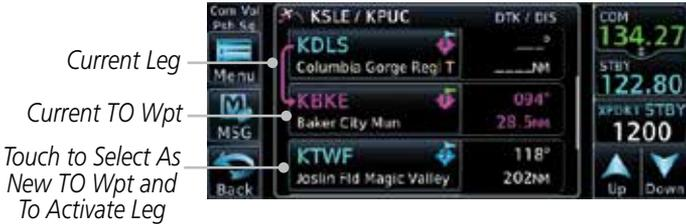
Figure 4-9 Active Flight Plan Activate Leg Option
