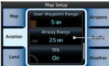
Figure 8-27 Map Setup For Airway Range
