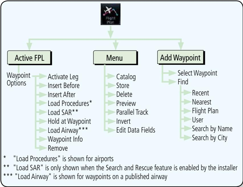
Figure 4-1 Flight Plan Functional Diagram
