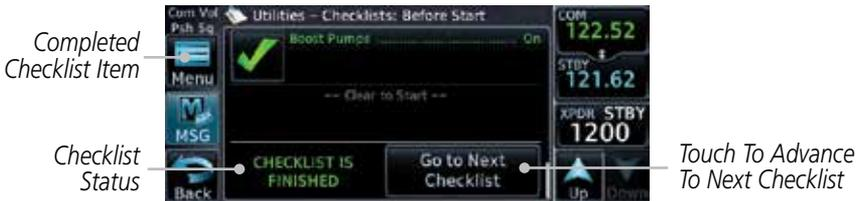
Figure 14-54 Checklist Completion
