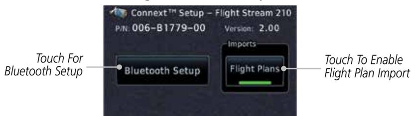
Figure 15-63 Connex Setup for Flight Stream 210
