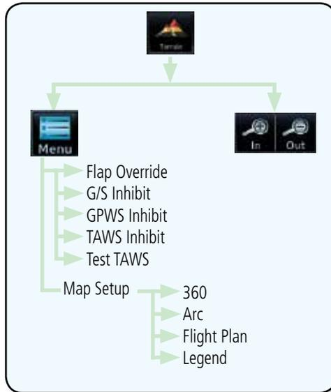
Figure 10-32 TAWS-A Page Functional Diagram
