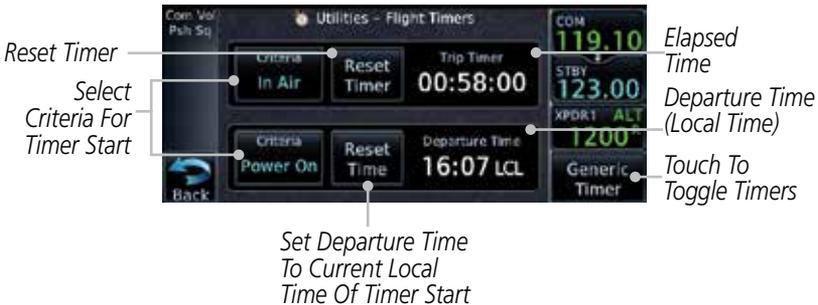
**Figure 14-12 Utility Flight Timers Page (Trip/DEP Timers)**
