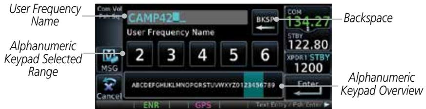
**Figure 3-21 Select a Name for the New User Frequency**
