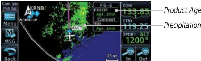
Figure 11-62 Connex Precipitation Data
