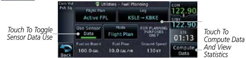
Figure 14-33 Utility Fuel Planning Page Showing Edit Input Data (Flight Plan Mode)
