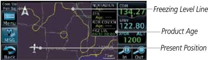
**Figure 11-25 Freezing Level**
