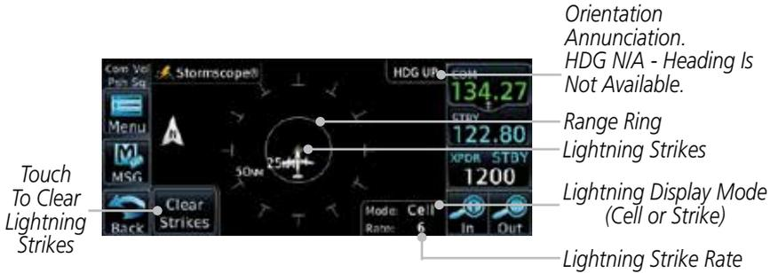
**Figure 11-45 StormScope Display (360° Display View Shown)**
