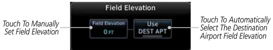
Figure 9-24 TCAD Traffic Field Elevation Selection
