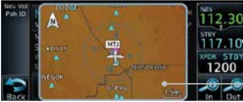
VOR Frequency Inserted Into Standby Window. Touch To Flip/Flop Freqs
